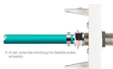
4. At last, screw the wired plug into Satellite socket accessory.
